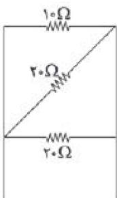
$$\frac{1}{R_{eq}} = \frac{1}{10} + \frac{1}{20} + \frac{1}{20} \Rightarrow \frac{1}{R_{eq}} = \frac{1}{5} \Rightarrow R_{eq} = 5\Omega$$
